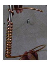
Notice the last turn (at the bottom of the pic) is straightened up so it comes back on itself, ready for the changeover.
