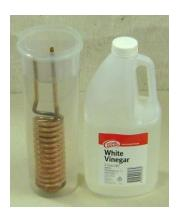
If you have a taller soaking container and can cover the tail ends with vinegar so the coolant path gets filled and cleaned too. Keep the coil vertical until it is filled with vinegar, to make sure all the air bubbles have been flushed out of the coolant path.
