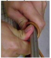
Keep the original angle between the tube and the mandrel until you get most of the way through the first turn, then start changing the angle towards 90 degrees.
