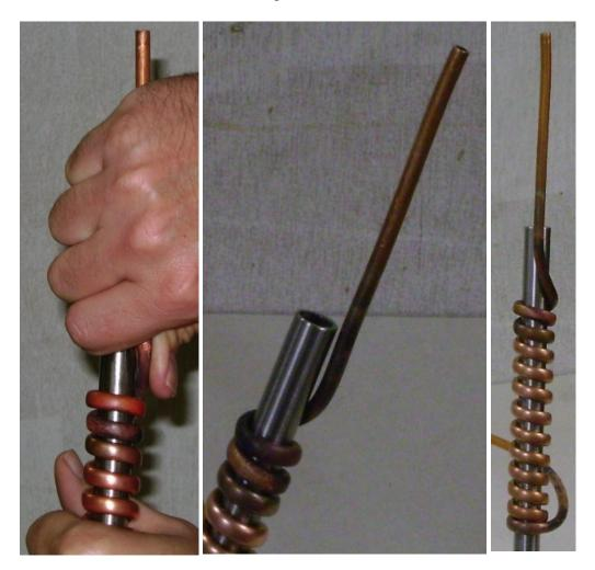
The aim is for the outer mandrel to be able to easily slide over the tail and inner coil.
