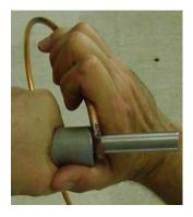
Having a roughened surface on this short outer mandrel helps to get a good grip. It may help to clamp the left hand end of the inner mandrel in a vice for this step.
