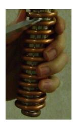
Then, if the outer coil is evenly spaced but is also still slightly shorter or longer than the inner coil, you can adjust the outer coil length by firmly (but carefully) grabbing both ends and pulling or pushing it. Be careful, it is easy to overdo it. You might want to put the outer mandrel back in to do this.
