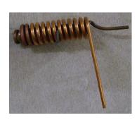
Remove the mandrel and re-anneal the last 1/8 of the last turn of the outer coil, and the 40 mm section of the outer tail immediately coming off the last turn of the coil.
