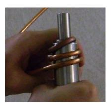
Once you have enough turns for you to be able to get a firm hold on the wound end (about 3-4 turns), then exchange the short outer mandrel for the long outer mandrel.
