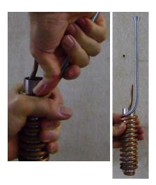
Remove the bending spring and mandrel, re-anneal the bottom half of the new bend.
