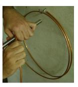
Holding it all as tight you can, and keeping as much tension on the tube as you can, pull the hand holding the tail down and around the mandrel, keeping the angle between the tube and the mandrel. Use your thumb as the pivot point.
