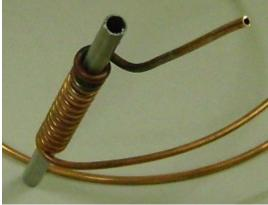
Remove the mandrel and re-anneal the new bend down to the first turn of the coil. Re-insert the mandrel and slide it up so about 75-100 mm is sticking out of the tail end of the coil. Work the tail to be as close a fit to the mandrel as possible.
