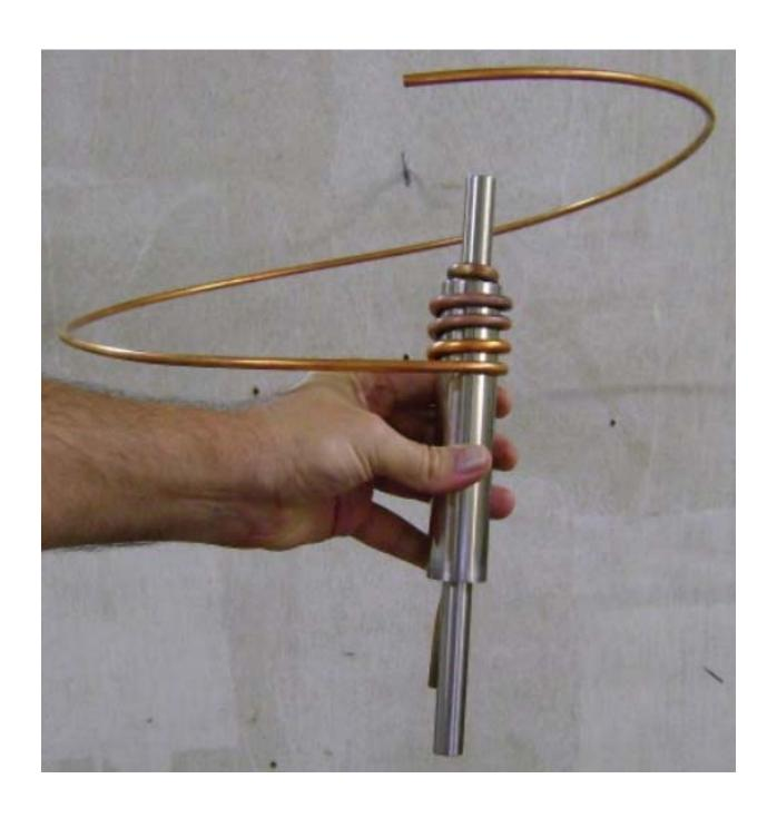
Swap sides and hands back, and continue winding the outer coil. This last section of winding is the easiest of all.
