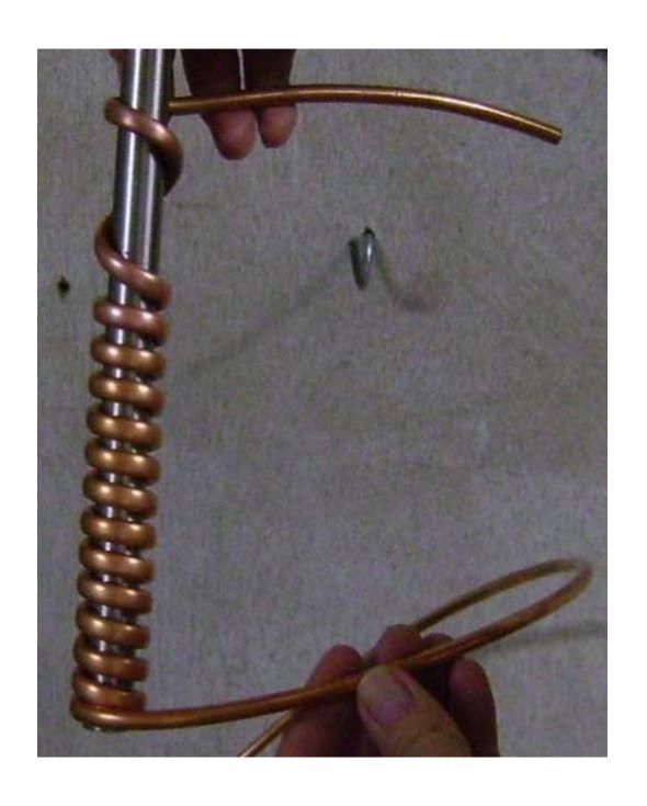
Notice the last turn (at the bottom of the pic) is straightened up
