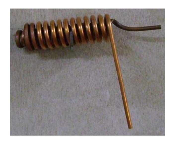
Remove the mandrel and re-anneal the last 1/8 of the last turn of the outer coil, and the 40 mm section
