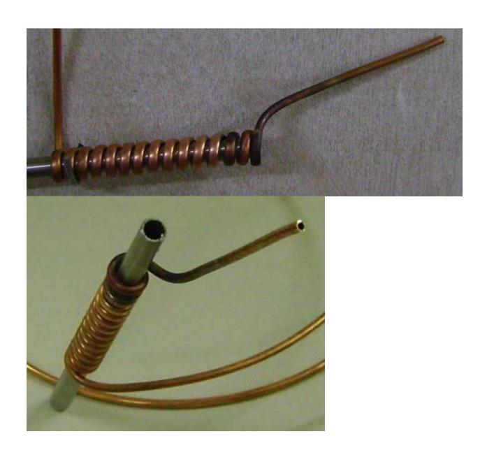
Remove the mandrel and re-anneal the new bend down to the first turn of the coil. Re-insert the mandrel and slide it up so about 75-100 mm is sticking out of the tail end of the coil. Work the tail to be as close a fit to the mandrel as possible.
