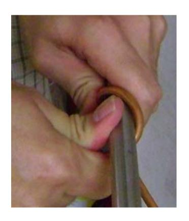
Keep the original angle between the tube and the mandrel until you get most of the way through the first turn, then start changing the angle towards 90 degrees. Swap sides and hands, and continue the wind until you have a full turn.
