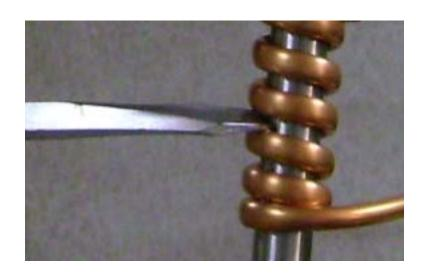
Remove the mandrel. Re-anneal the 40-50 mm section of the tail immediately coming off the first turn. Re-insert the mandrel to level with the bottom of the first turn (bottom right of pic).
