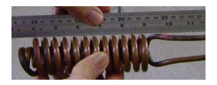
After you have used the mandrel and bending spring to adjust the outer tail, you may need to work the tail by hand a little further towards the centre of the condenser, to get it in the right position to fit easily and evenly inside the column. Do this carefully. I find it better not to re-anneal for this last small adjustment.
