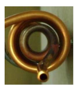
If you have some excess tube as you get near the end of the wind, then bunch up the coils a bit and use up that extra tube, (but make sure you leave enough unwound tube for the tail). You can adjust the spacing afterwards.
