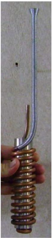
Remove the bending spring and mandrel, re-anneal the bottom half of the new bend.
