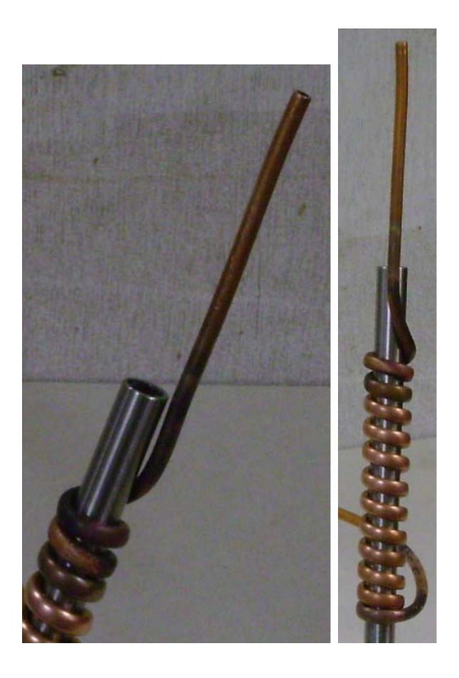
The aim is for the outer mandrel to be able to easily slide over the tail and inner coil.
