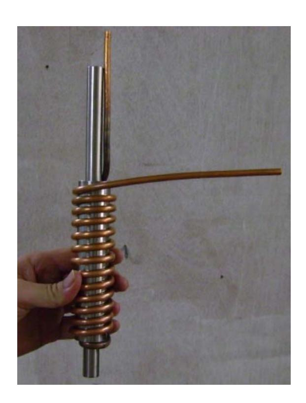
As you get towards the end of the outer coil, keep an eye on the alignment between the inner tail and where the outer tail will end up. You need to avoid the inner and outer coils or tails crossing and touching in the finished condenser.
