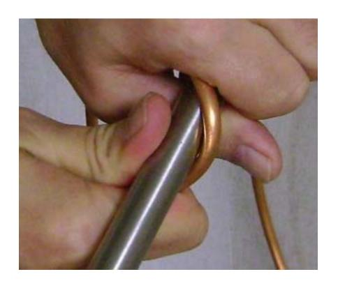
You will get some degree of flattening of the tube as you wind the coils, mainly on the inner coil. This is not a problem, as long as it is only minor.
