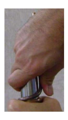
The outer tail has to be flush with or slightly inside the outside line of the outer coil, so that the whole condenser can slide easily and evenly inside the column.
