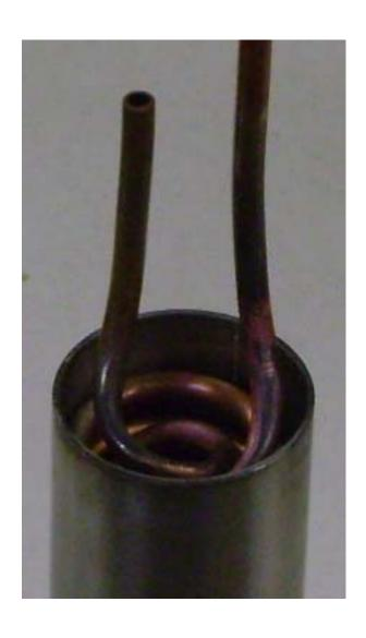
Finally, make sure the outer coil is straight. Adjust if necessary.
