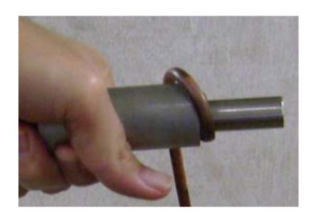
The first turn after getting onto the outer mandrel is difficult, and this is one of the danger points for kinking. But just persist with it a little bit at a time. Try doing this turn in 3-4 steps, rather than all at once.
