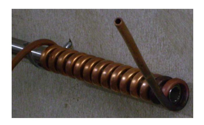
Use the bending spring to turn the tail upwards, towards parallel with the coil axis. Pivot around your thumb.
