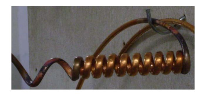
Re-insert the mandrel. Alternatively compress, tighten, and align the widely spaced turn or two at the top of the coil, in steps, and generally work it until it is matched up with the rest of the coil. You may need to re-anneal this section of coil about half way through this process.
