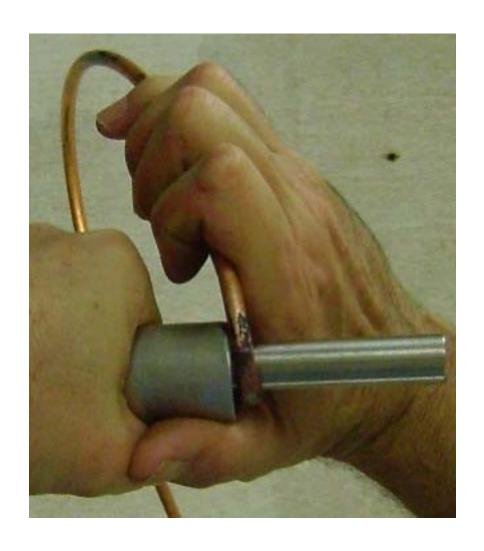
Having a roughened surface on this short outer mandrel helps to get a good grip. It may help to clamp the left hand end of the inner mandrel in a vice for this step.
