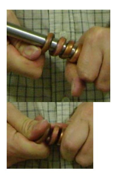
Re-insert mandrel, and use a twisting motion of the screwdriver to evenly space the coil turns (except that last one, at the bottom).
