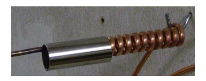
Check the inner coil is straight overall, and carefully adjust if necessary. It should be fine, but check because you can't adjust it
