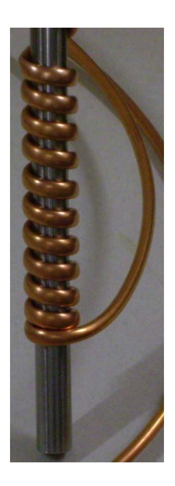
Remove the inner mandrel. You may have to loosen the coil a little by gently twisting it against the direction of the wind. (Hand on left of pic is twisting up, hand on right is twisting down.)
